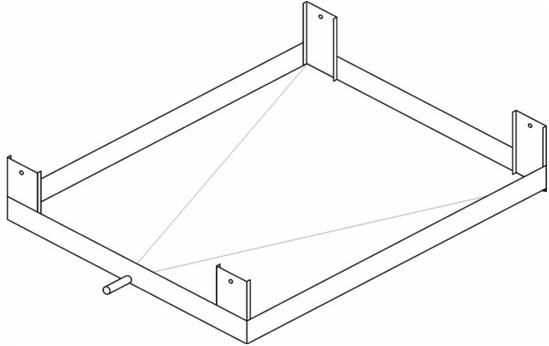
**A-COIL DAMPER KIT (wood furnace)**
